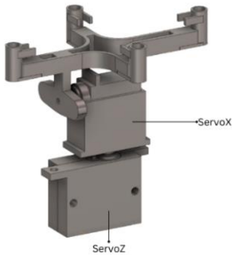
Fig. 5. Actuation mechanism of the proposed solar tracking prototype
