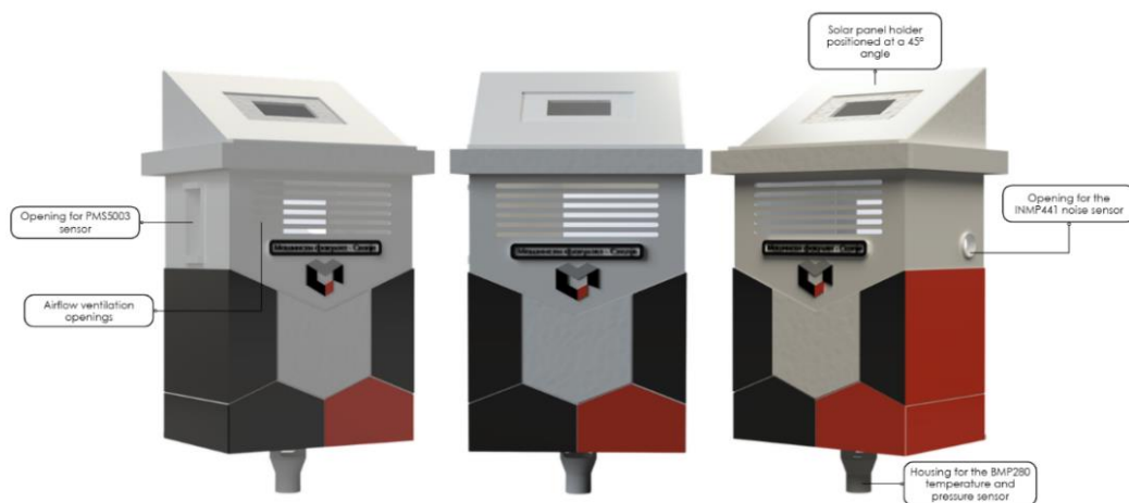
Fig. 7. Mechanical design of the 3D-printed sensor unit enclosure
