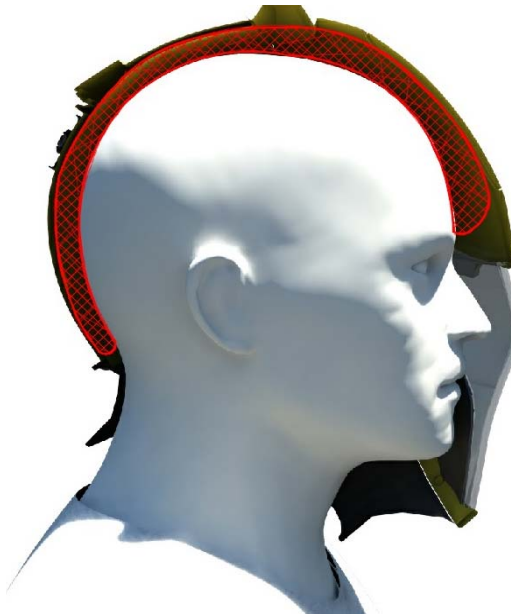
Fig. 18. Head inlay with polyurethane
