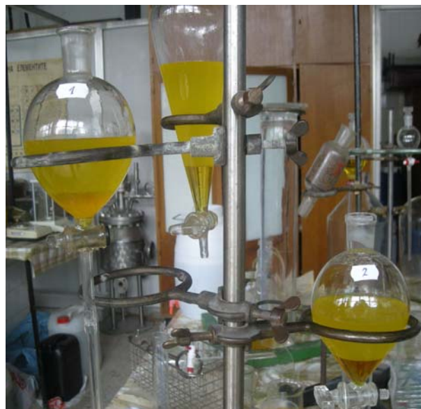
Fig. 2. Glycerol and esters phase separation
