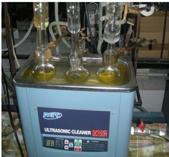
Fig. 3. Laboratory equipment for ultrasound-assisted biodiesel production
