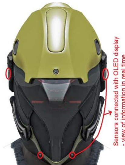
Fig. 13. Sensors on the side of the helmet
