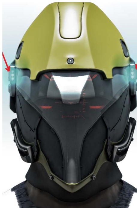
Fig. 15. LED lights placed on both sides
