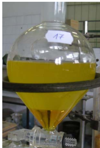
Fig. 4. Methyl esters (upper) layer and glycerol (lower) layer in the separating funnel
