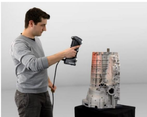
Fig. 2. Creaform HandySCAN handheld 3D laser scanner [4]
