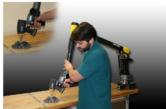
Fig. 4. Arm based 3D scanner and probing system [4]
