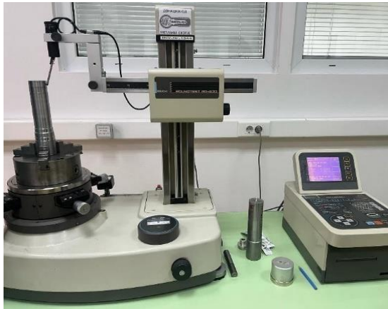
Fig. 1. Mitutoyo Roundtest RA-400 instrument used for cylindricity measurements
