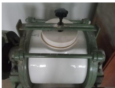
Fig. 4. Porcelain mill with balls
