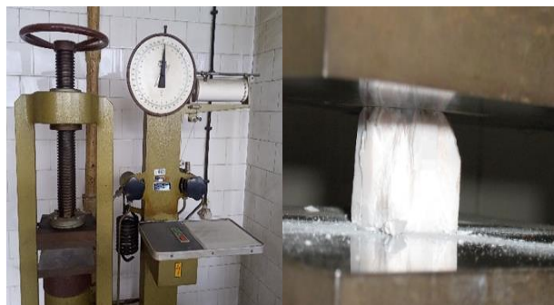
Fig. 5. Pressure strength testing
