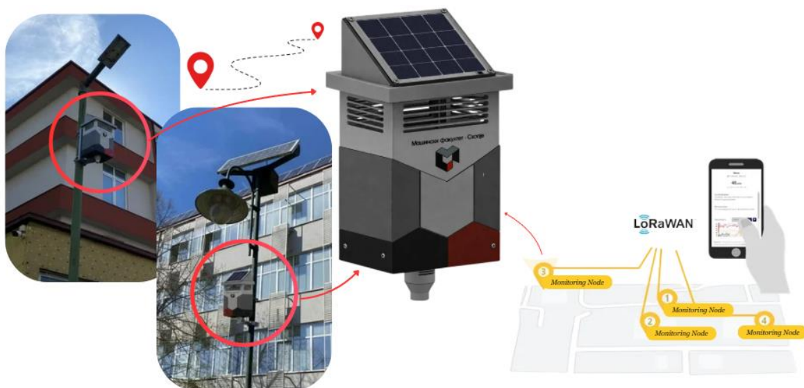
Fig. 1. Campus deployment concept of the IoT environmental monitoring system
