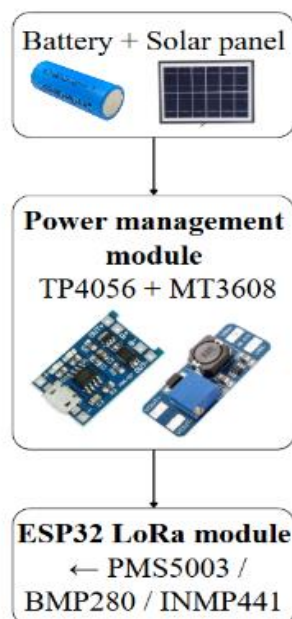
Fig. 8. Power supply concept of the proposed IoT sensor unit
