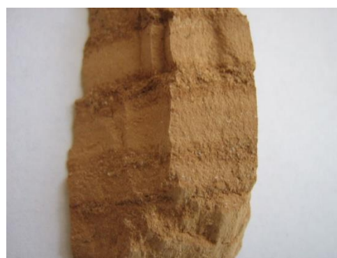
Fig. 15. Thermally treated diatomaceous earth sample at 800^{\circ}\text{C} for 2 hours (in an oxidizing atmosphere)
