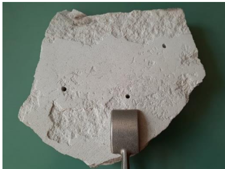
Fig. 10. Perforation of the material at different depths for the placement of the thermal sensor
