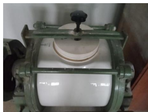
Fig. 4. Porcelain mill with balls
